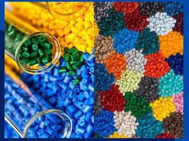
Coloured masterbatches, characterized by a high pigment rate, exhibit impeccable dispersion, high heat resistance light fastness, superior performance, and vibrant coloration. This product group, comprised of coloured densified masterbatches, is specifically formulated for colouring raw materials such as LDPE, HDPE, PP, PE, PVC and PET. These materials are utilized in film production, PP raffia, and plastic bag manufacturing through methods such as pouring, inflation, and extrusion.
